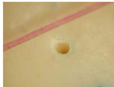
Bone ablated by laser. The pink line is an optical fiber.
