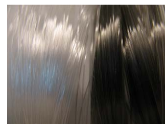
Carbon coated fibers with their characteristic dark grey color.
